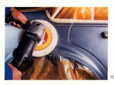
Leave 3M™ Soft Edge Foam Masking Tape in place when buffing to help prevent compound and polish sling from entering jamb areas; thereby saving time during the clean-up step.
