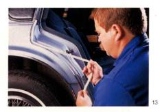
To remove, slowly pull up and away from painted surface. The "soft edge" from 3M™ Soft Edge Foam Masking Tape virtually eliminates rework due to unwanted tape lines.
