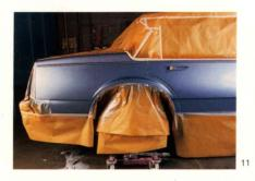
Mask as usual and refinish the repair. 3M™ Soft Edge Foam Masking Tape will help protect jambs from paint overspray, while sealing in dust and other contaminants.
