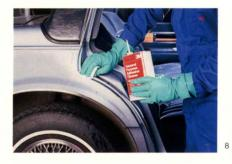
Clean area to remove dirt and contaminants where 3M<sup>™</sup> Soft Edge Foam Masking Tape is to be applied. Use soap and water followed by 3M<sup>™</sup> General Purpose Adhesive Cleaner (Part No. 08984) to assure proper adhesion.
