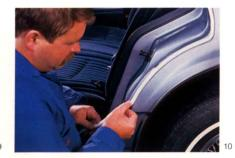
Apply to jamb area leaving a 3/16-inch set-back from outer edge. Allow 3M™ Soft Edge Foam Masking Tape to lay into area (DO NOT stretch) as you firmly press in place. Run thumb in reverse direction over entire length of 3M Soft Edge Foam Masking Tape applied. This allows a better adhesion by reducing any excess tension.
